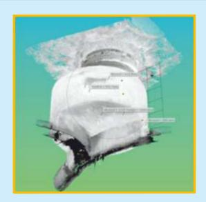
The 3-D laser survey and the digitalising of the gathered data are the premises for producing the bespoke rehabilitation FLEXLINER.
