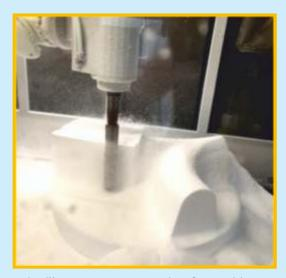
The Styrofoam model has been made with the scanned data and will serve as a negative for making the FLEXLINER and for strengthening it when pouring the grout.
