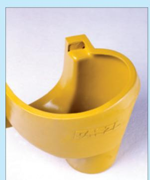
The big advantage which is given with the IPK, is that it can be fitted easily in an existing manhole. It's special construction produces a cyclone type stream of the sewage waters. Therefore the flow energy is reduced.
