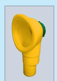
The Inside Drop can be fitted in new - as well as in existing-manholes. It is mounted with V2A screws and a seal on the inside wall of a manhole ring and takes pipe connections up to DN 250 (Inside Drop DN 200) and respectively 300 mm (Inside Drop DN 250).
